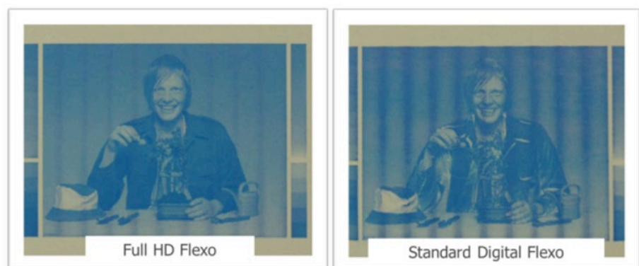
Figure: Typical fluting visibility for Full HD Flexo printing (left) and standard digital Flexo printing (right).
