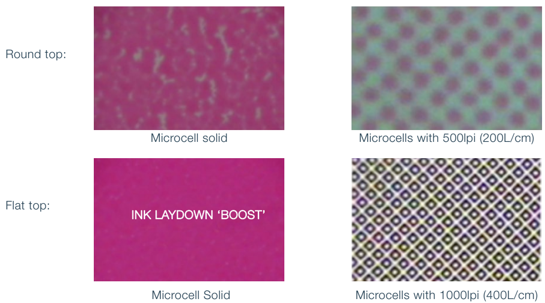
Figure: Print results with round top and flat top microcells (left) as well as an image of the corresponding flexo plate surface (right)
