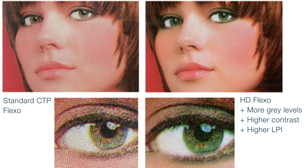
Figure: Comparison of standard and HD flexo print quality
